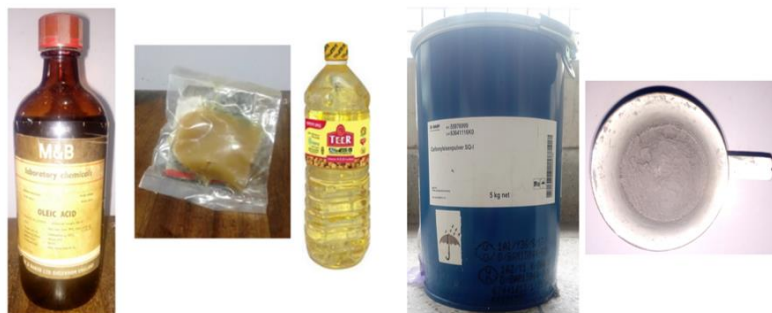
Figure 4. Oleic Acid, Grease and Soybean Oil (Left), CI Powder Container and CI Powder (Right)
